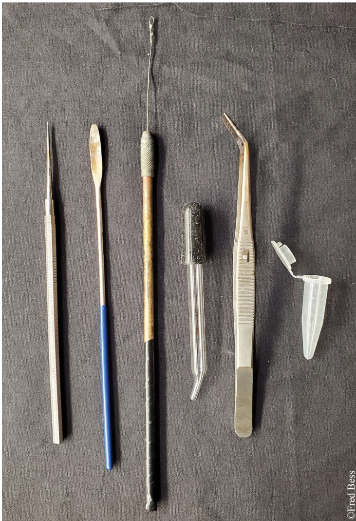
Tools used: left to right: Dissecting needle, Micro-spatula, Inoculating needle, Eyedropper, 6 -inch tweezers, Centrifuge tube for seed sterilization.
