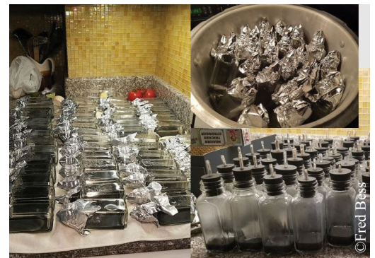
Flasks on the left, cooling after sterilization, on the upper right, in the pressure canner, and lower right ready to load into the canner.
